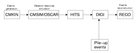
Fig.5. Complete cycle of the CMS event generation/reconstruction.
