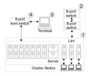
*Fig.2. KCLC layout: 1 – server and nodes; 2 – two ethernet switches; 3 – terminal; 4 – kvm switch.*
