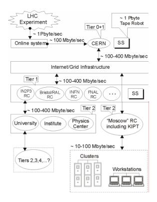
Fig.1. Hierarchy of Grid structures for LHC experiments.
