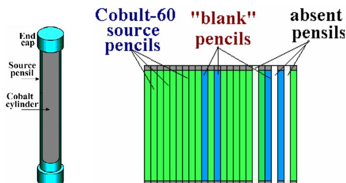
*Figs.2. (a) and (b). (a) Source pencil constructions.
