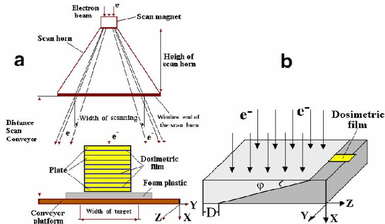
*Figs. 7a,b. a) Electron beam and irradiated dosimetric stack geometry. Arrangement of a stack plates interleaved with dosimetric films on moving conveyor irradiated with EB and triangular scanning. Axis X - direction of EB incidence, axis Y - direction of EB scanning, axis Z - direction of conveyer motion.*
