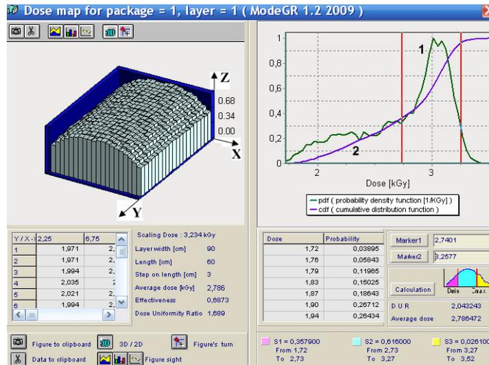
Fig.4. Left Graph: 3D view of the depth dose distributions of Gamma ray (Dose Map, along layer length (axis Y) and along layer width (axis X) in graphical and tubular forms for the 1<sup>st</sup> layer in 1<sup>st</sup> package. The dose value is integrated along layer thickness (axis Z). Right graphs: Cumulative distribution function – cdf (curve 2), and Probability density function in 1/kGy – pdf (curve 1).
