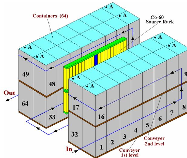
Fig.3. Sequence of irradiation in a flat panoramic  $\text{Co}^{60}$  source rack, multipass, two direction, multiposition. The 64 aluminum containers with product are moved around the  $\text{Co}^{60}$  source rack on a conveyor 8 passes at two levels. Point “A” is a fixed point on the side surface of the process load, which passes through the irradiation room on both sides of the  $\text{Co}^{60}$  source rack from position 1 to position 64.
