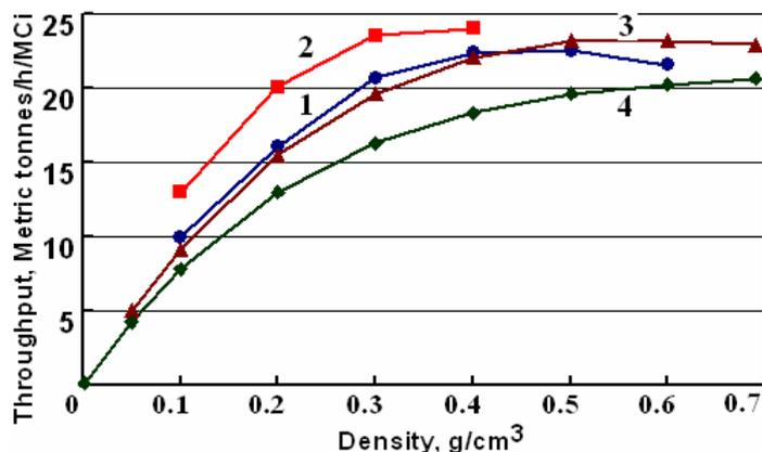
Fig.6. Curves 1 and 2 - dependence of product mass throughput at absorbed dose 1 kGy on product density for two irradiator designs by MDS Nordian, Canada. Curve 3 was calculated at density  $0.002\text{g/cm}^3$  of the metal layer, curve 4 - at density  $1\text{g/cm}^3$  of the metal layer
