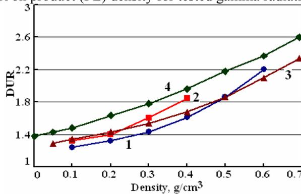
Fig.4. Curves 1 and 2 – Dependence of dose uniformity ratio (DUR) on product density for two different irradiator designs by MDS Nordion, Canada. Curves 3 and 4 – simulation results for dependence of DUR on product (PE) density for tested gamma radiation facility
