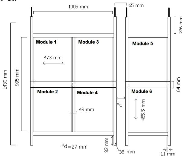
Fig.1. Arrangement of source modules in the NCRRT panoramic source rack with active cobalt-60 source pencils
