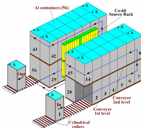
Fig.3. Sequence of irradiation in a flat panoramic  $\text{Co}^{60}$  source rack, multi-pass, two direction, multi-position. "A" is a fixed point on the side surface of the process load, which passes through the irradiation room on both sides of the  $\text{Co}^{60}$  source rack from position 1 to position 56, with four passes on each side of the source.
