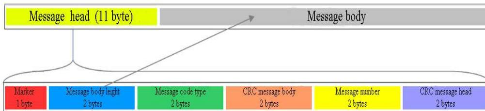
Fig. 3. The frame structure.
