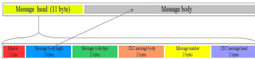
*Fig. 3. The frame structure.*
