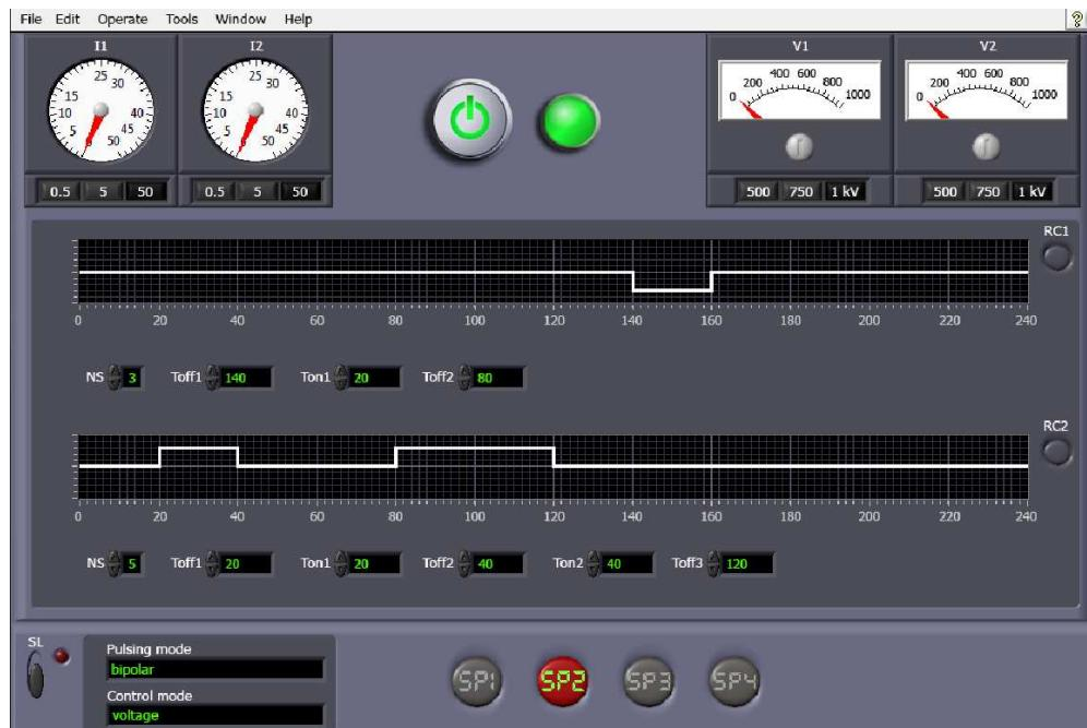
Fig.4. The management subsystem of AC pulsed ion source
