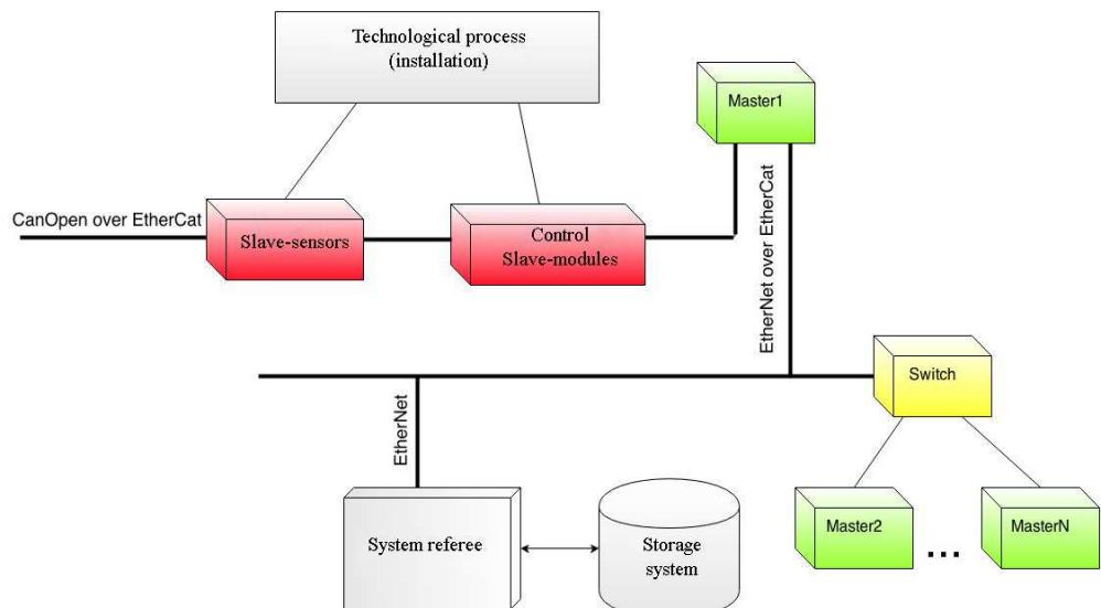
Fig.1. System with split-architecture management - PLC-technology
