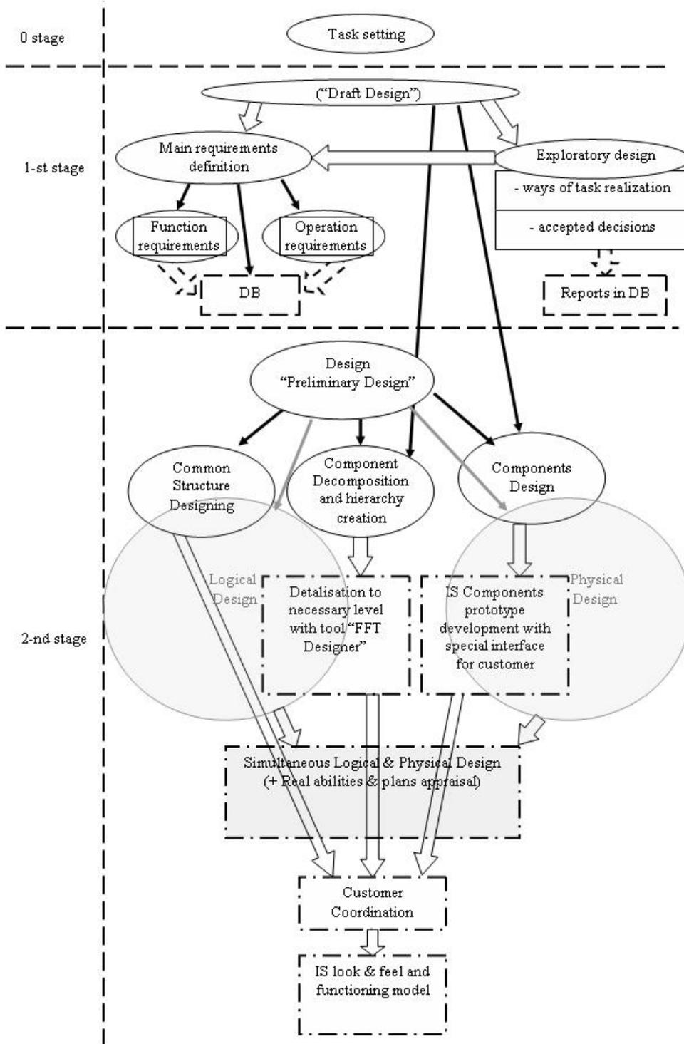
Figure. 1. Standard and modern "Draft & Preliminary Design" integration
